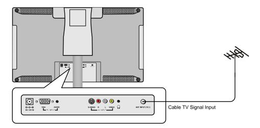
After connection, turn on the power of the unit. Then press the INPUT button to shift to TV mode.
